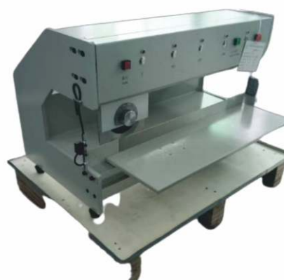
TOKii-400DPM Knife Splitting Machine 0-400 mm
