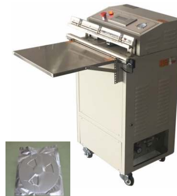
TOKii-VP60030 TOKii-VP60031 Vacuum Sealing and Nitrogen Purge, meets Class 100.
