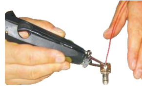
Model: SI 1R (80 W) & Model: SI 2R (250W) Quick instant heat transfer local heating without damage to insulation of connector.
