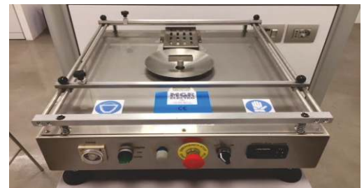
Mini Wave for Selective Area Helps in soldering or Reworking, different kinds of nozzles as per customer's requirement is available.
