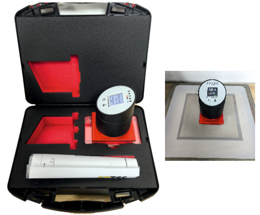
Swiss SEFARTensocheck 200 Digital mesh tension meter
