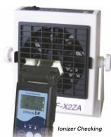
Handy Charge Plate Monitor Model STATIRON DP
