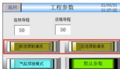
5.10 In the red picture box, there is the switching button of forward feed tin mode/back feed tin mode cleaning mode
