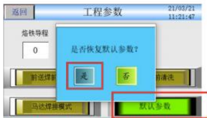
5.12 In the red box is the factory setting parameter recovery button. Press the default parameter button first, then jump out of the dialog box as shown in the figure above, and then restore the factory parameters. Please use this function with caution, as this function is used in the case of abnormal operation of the equipment, otherwise all the original processing data will be lost and need to be set again
