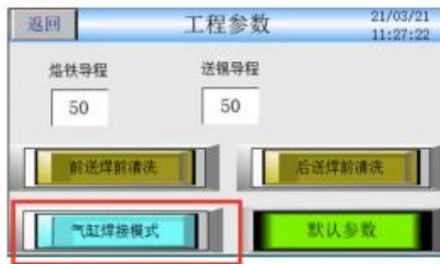
5.11 In the red frame is the switch button of cylinder welding mode/motor welding
