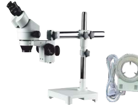
TOKii-SM0745EA Stereo Microscope with Extended arm with LED Source
