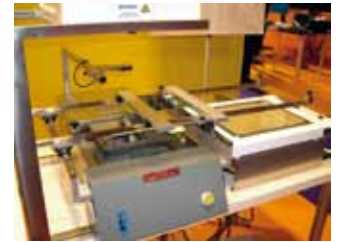
MV500 Mini Wave With up / down and x, y translation table system
