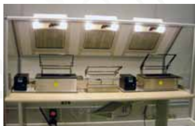
Example of a full degolding / fluxing / tinning station with pantograph SOLDER BATH WITH PANTOGRAPH
