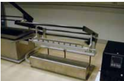
FLUX TRAY: fluxing station with pantograph, accepts the same component holder tool as the robot
