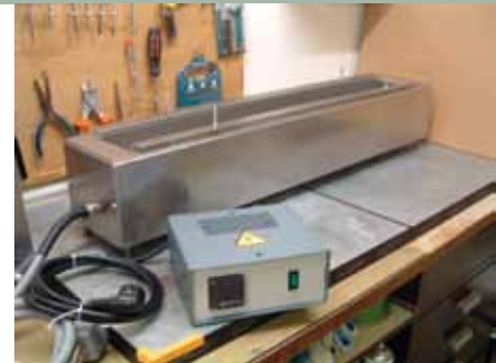
LONG CRUCIBLE: example of a long solder bath 1.20 m
