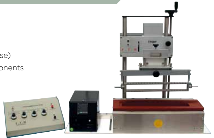
TP60P : Tinning Machine with Solder Bath
